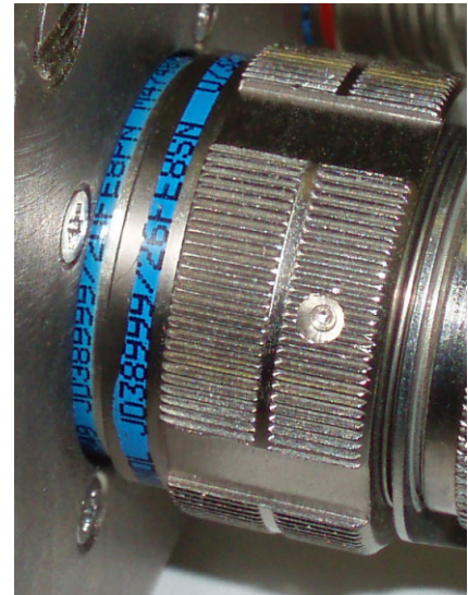
Red band covered – completely mated
