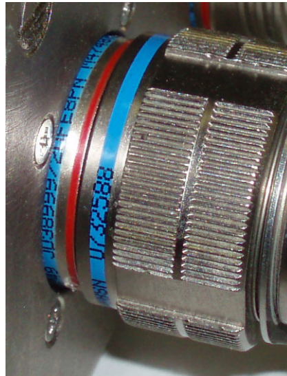
Red band exposed – not completely mated
